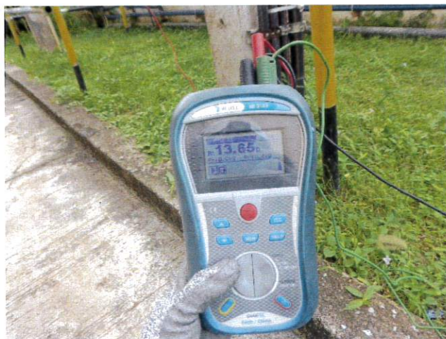
GROUNDING RESISTANCE TEST
