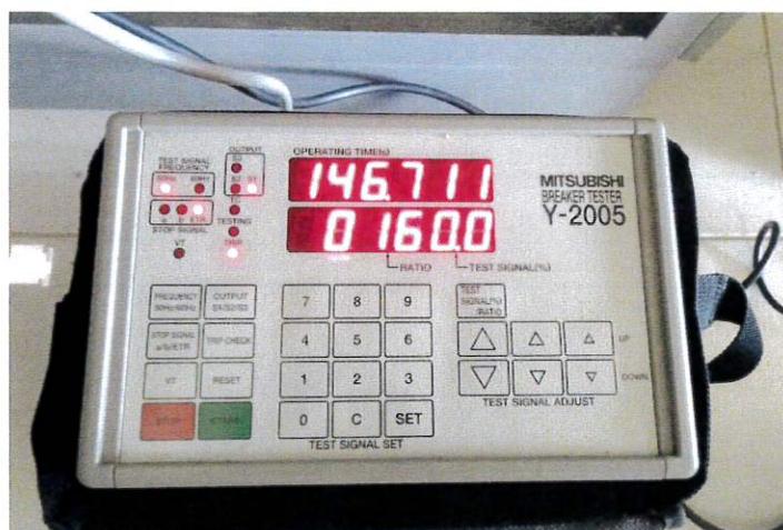
ACB TRIP UNIT TEST
