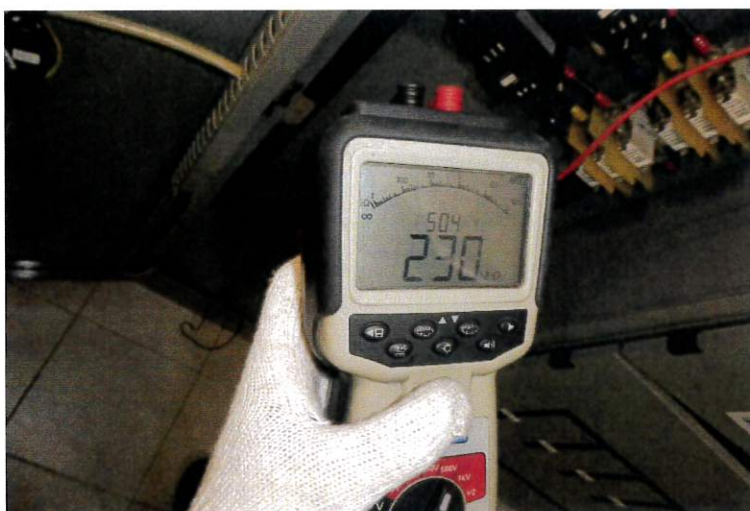
INSULATION RESISTANCE MEASUREMENT
