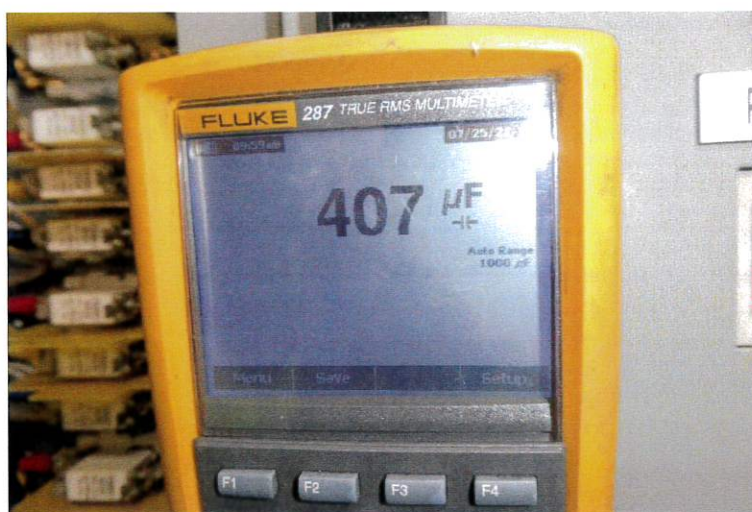
CAPACITANCE MEASUREMENT
