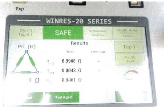
20A Winding Resistance Meter
