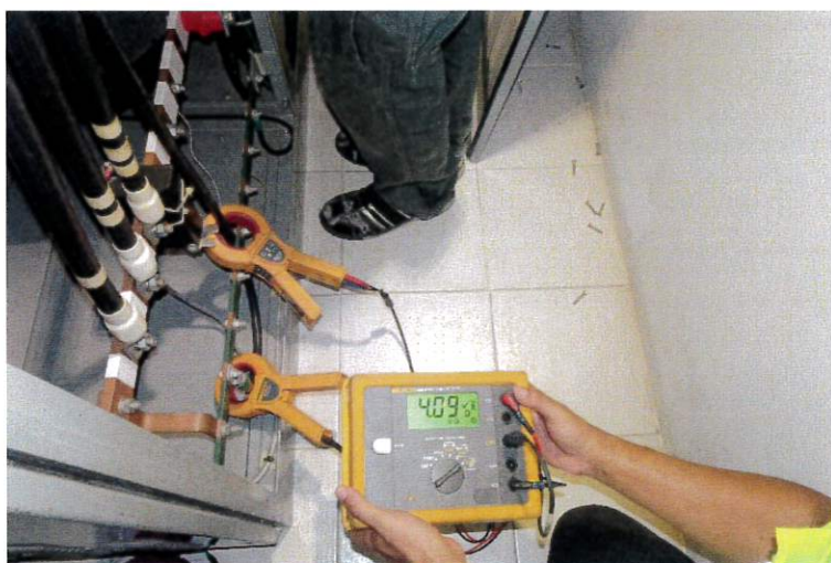
GROUNDING RESISTANCE TEST
