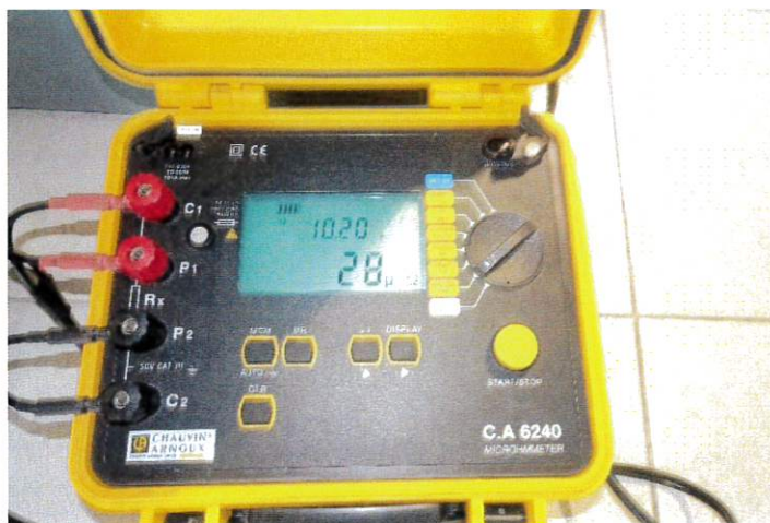
CONTACT RESISTANCE TEST
