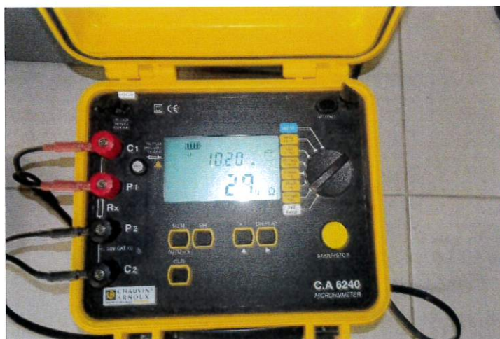
CONTACT RESISTANCE TEST
