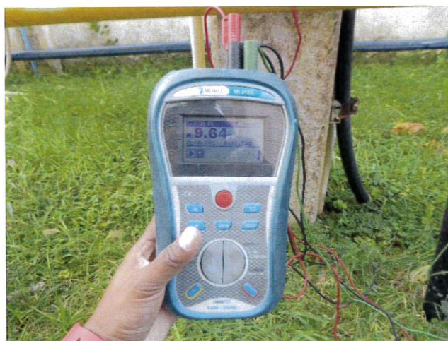
GROUNDING RESISTANCE TEST
